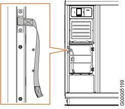
Fig. 10 Roller bed handling
