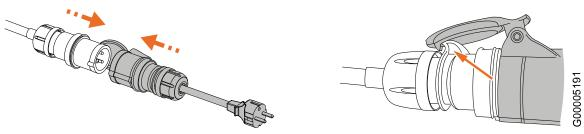
Fig. 25 Connect an adapter
