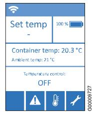
Fig. 38 Temperature control is turned off
