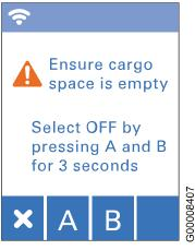
Fig. 37 Turn temperature control off
