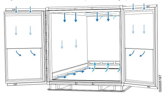
Fig. 4 Schematic view of the internal airflow
