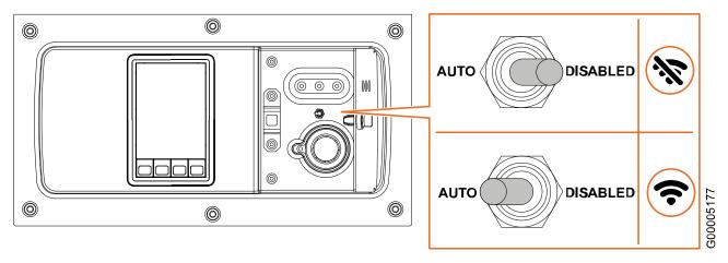
Fig. 40 Connectivity switch
