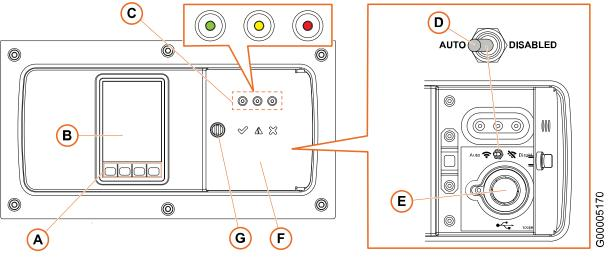
Fig. 33 Overview of the display unit
