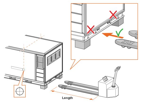
Fig. 9 How to lift the container with an electric pallet jack (example: Releye RLP container)
