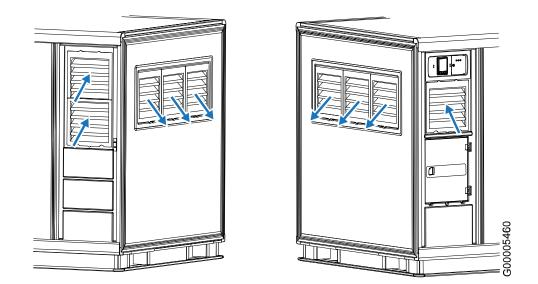
Fig. 5 Schematic view of the internal-external airflow transition (example: RelEye® RLP container)
