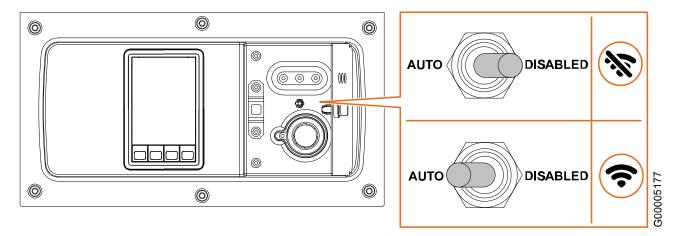
Fig. 42 Connectivity switch
