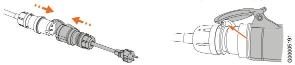
Fig. 27 Connect an adapter
