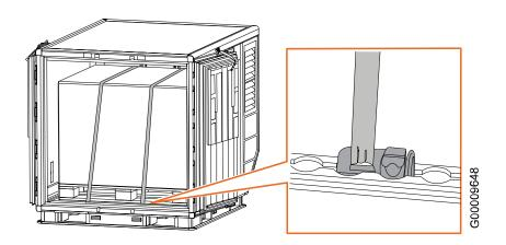
Fig. 22 Fasten and suspend cargo straps in the cargo space
