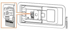
Fig. 23 Close, lock and seal the doors
