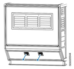
Fig. 6 Fan unit outlets in outboard panel
