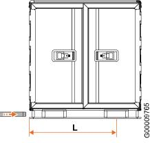
Fig. 10 Lift from the sides
