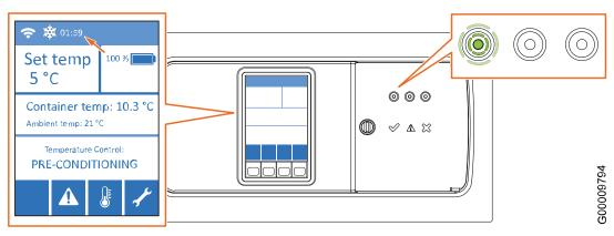
Fig. 15 The remaining pre-conditioning time
