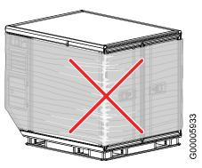
Fig. 33 Do not wrap the container
