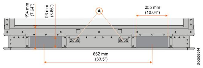
Fig. 9 Fork lift pockets and tie-down brackets
