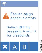
Fig. 39 Turn temperature control off
