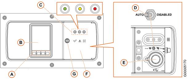
Fig. 35 Overview of the display unit
