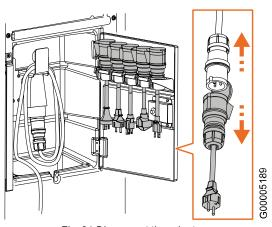
Fig. 31 Disconnect the adapter
