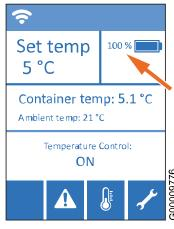
Fig. 37 The battery level
