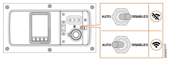
Fig. 40 Connectivity switch
