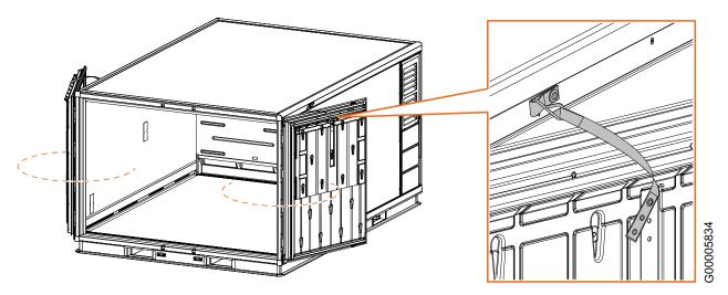
Fig. 15 Open and lock the doors in the opened position
