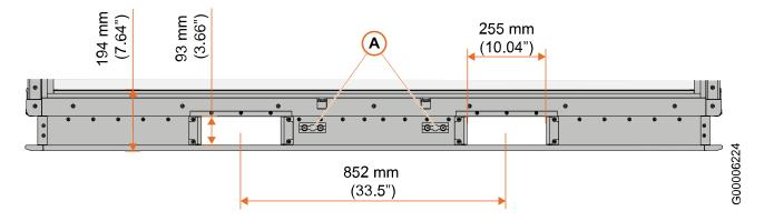
Fig. 8 Fork lift pockets and tie-down brackets
