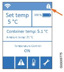
Fig. 42 Locked display
