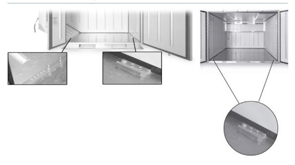
Figure 4 & 5 – Load the cargo on a pallet with 2cm spacing before securing the cargo to the tie-down brackets inside the container
