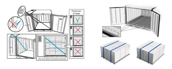
Figure 6 – Door straps are installed in all Envirotainer container doors to hold the doors open during loading
